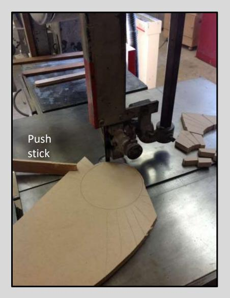
If cutting long stock, get help to hold up weight on the outfeed side of table.
