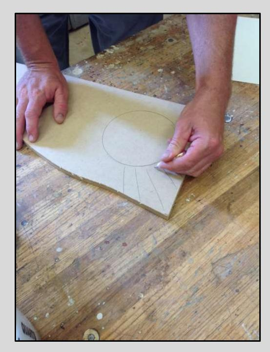
Hold stock down on table and move gently into the blade. Do not try to hold material in air, off of table.
