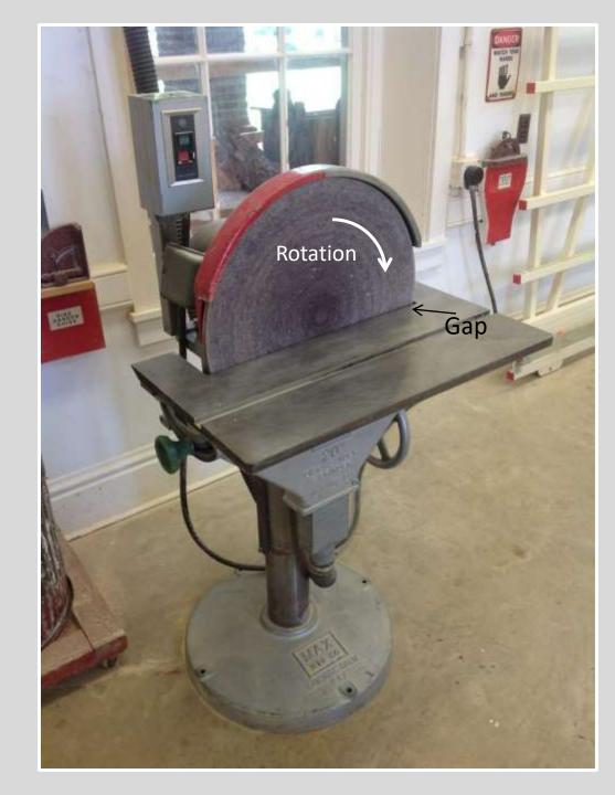
Small material can be sanded on the Disc Sander, but will require a backing board to be clamped to the table and close the existing gap.
