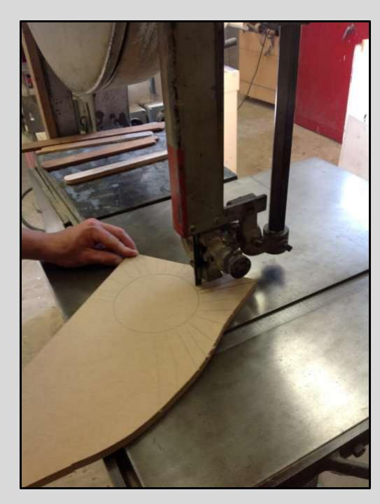
Now that plenty of relief cuts have been made, the operator makes a series of cuts to knock out large areas at a time. Again, these cuts need to be relatively straight to avoid twisting the blade.
