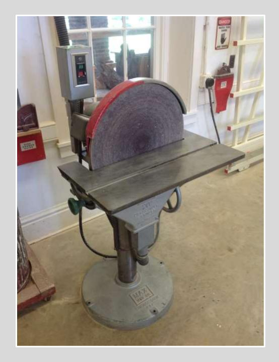
Check that material is not small enough to be pulled into gap between table and disc.
