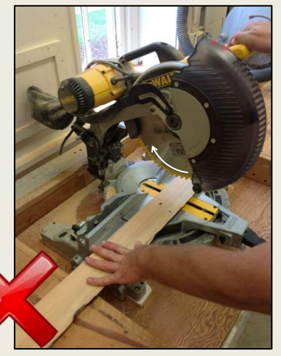
In this photo, the operator demonstrates how to safely cut a mitered edge. Rather than holding the wood at an angle, he has adjusted the angle of the blade.
