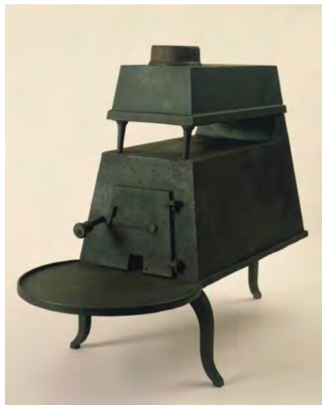
Wood stove with super heater. Cast iron. Pleasant Hill, KY. Courtesy of the Shaker Museum, New Lebanon, NY.
