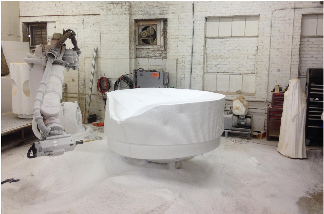
The KUKA robotic arm carving an enlarged rendering of Pill (from a foam block formerly part of an installation by Sabina Ott). Douglas Jonston built this robot from parts and was instrumental in making this happen.
