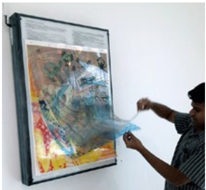
Flipping reproduced films of color separation in CMYK to visualize ink build-up in larger format on light box [below]
